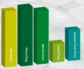
world. PE has high mould cost and is therefore only recommended for high quantities. The durability is very good, PE has limited possibilities to be recycled. There are a number of species of bacteria and animals that are able to degrade polyethylene. Open-Loop
